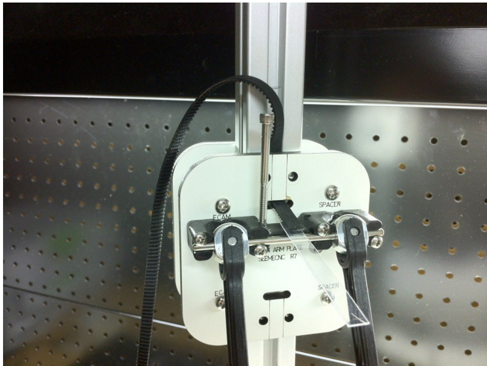
Routing the belt on a plastic "ramp".
