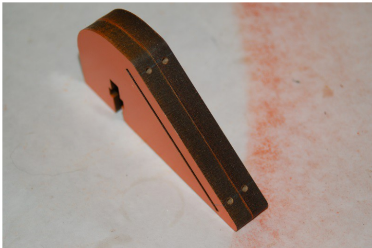
Fig. 16-15: Pilot holes for mounting the LCD panel.
