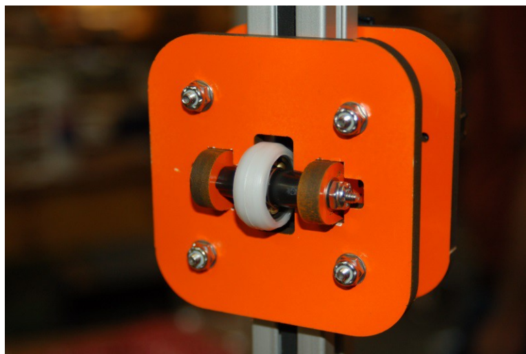
Fig. 7-25: Axle Support installed in the Cheapskate bearing assembly.
