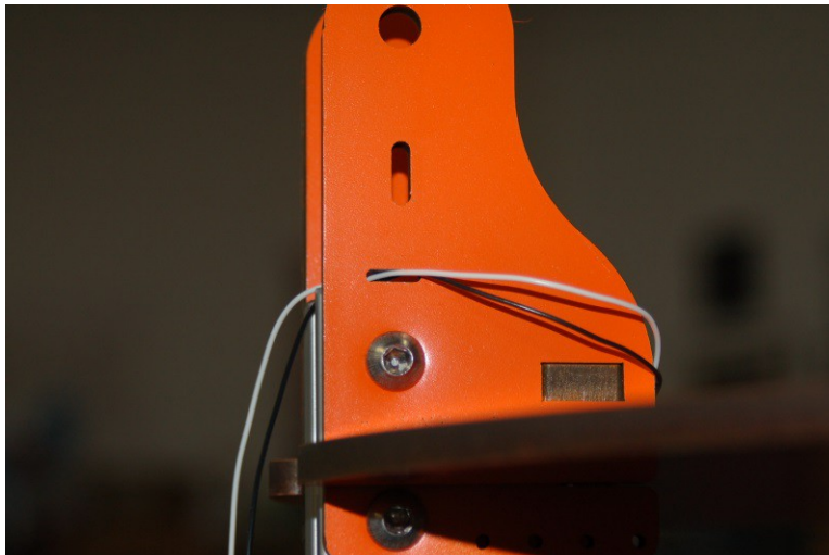
Fig. 6-2: Routing the end stop wires, step #2.
