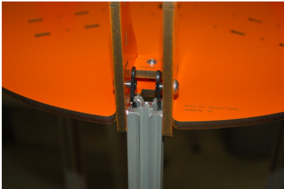
Fig. 5-1: Setting the Idler Mount into the tower extrusion.
