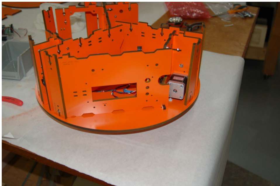
Fig. 2-32: Installation of the Support Panel
