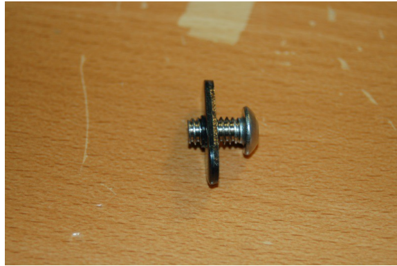
Fig. 3-2: T-Nut boss orientation.
