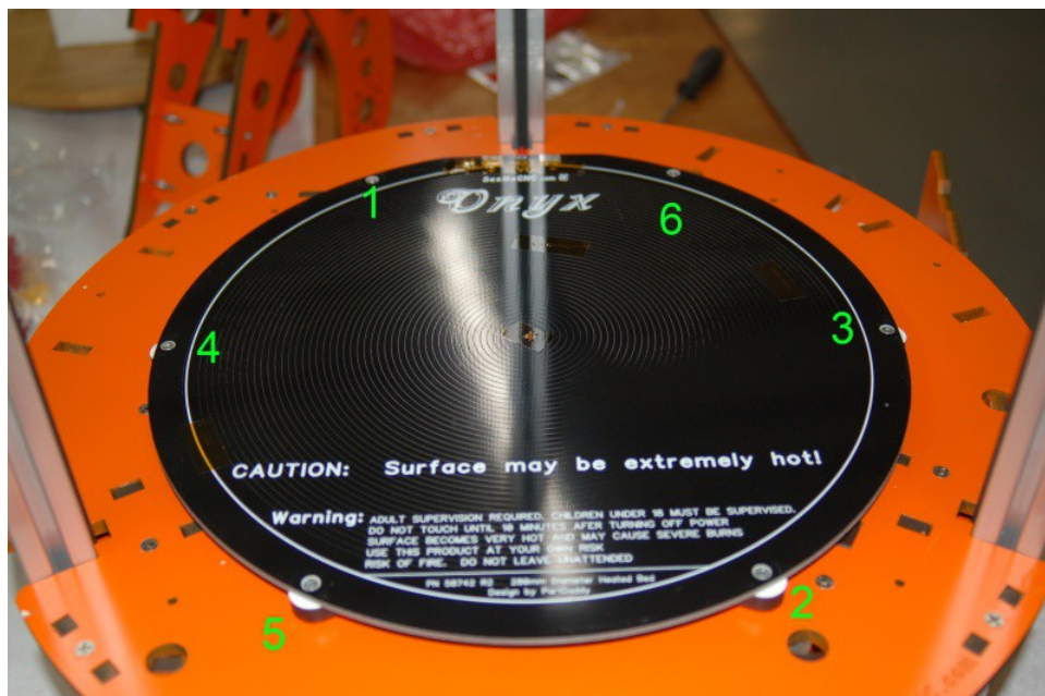
Fig. 14-10: Suggested fastener tightening pattern.
