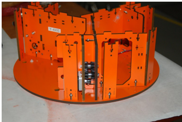
Fig. 2-31: Installing the Cover Brackets.
