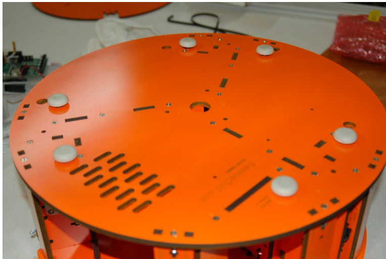
Fig. 2-40: Screws tightened and shoes installed.
