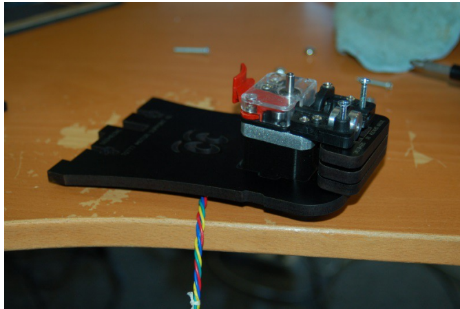
Fig. 11-13: Attaching the EZStruder to its mount.
