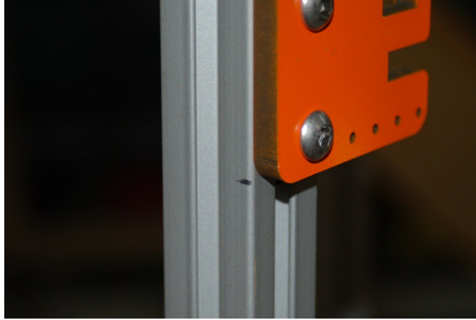
Fig. 4-2: Marking the bottom of the Idler Mount.
