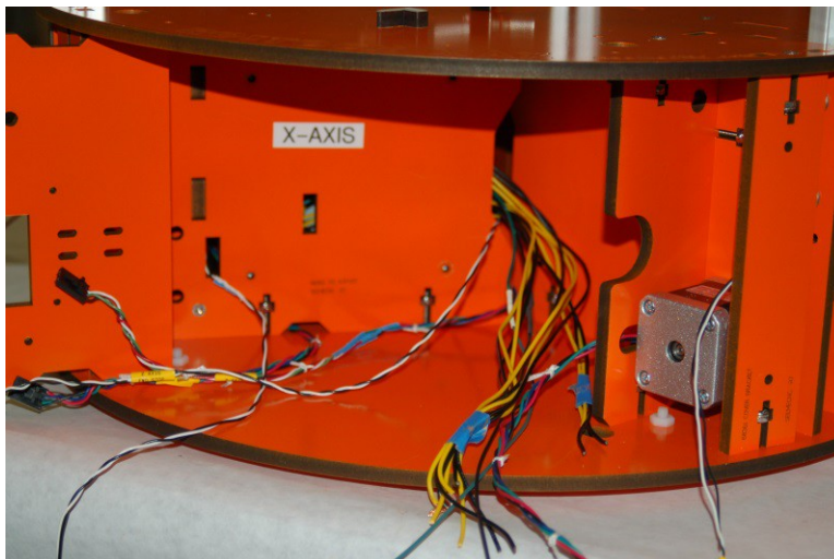
Fig. 13-4: Power wires routed to the electronics bay.
