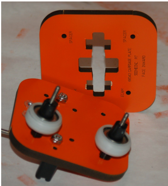
Fig. 7-14: Carriage Plate showing the spacer mounting holes.
