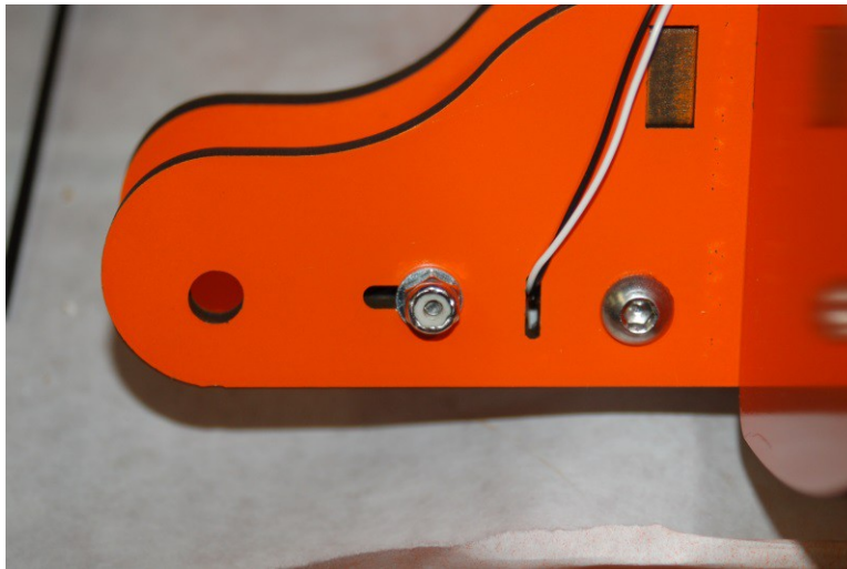
Fig. 8-9: The belt tension adjustment.
