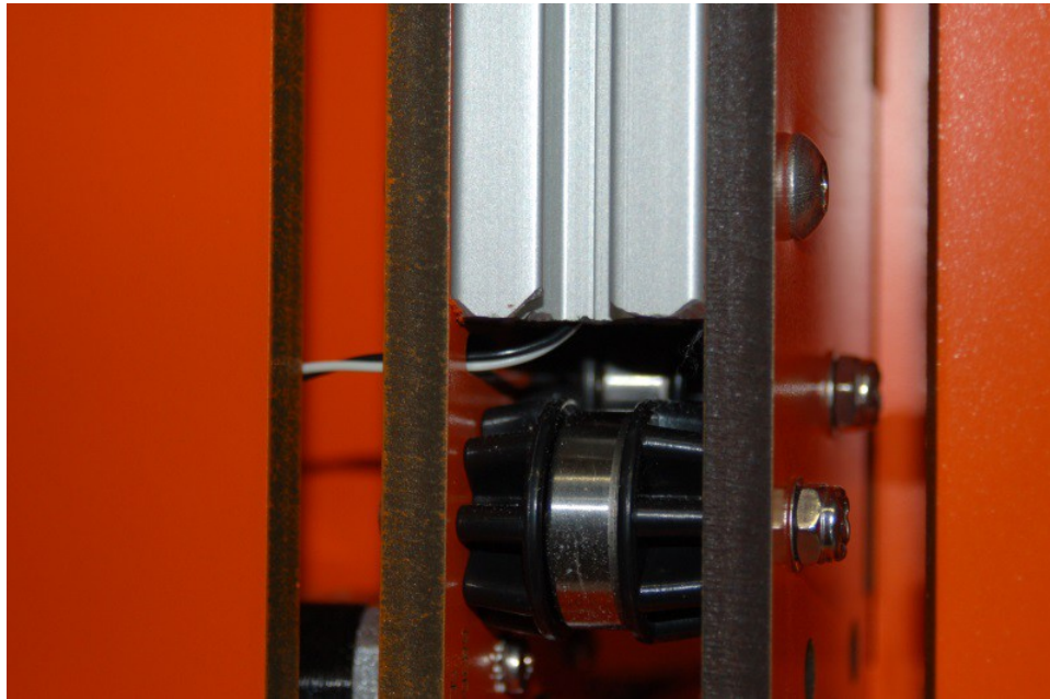
Fig. 6-5: Routing the end stop wires through the Tri-Support. (Step #4)
