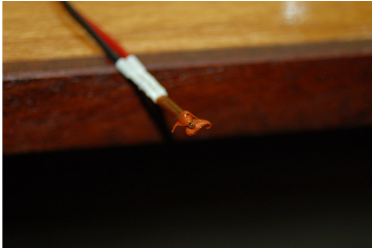
Fig. 15-12: RTV applied to the thermistor sides.
