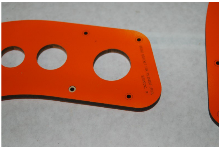
Fig. 11-2: Extruder bracket with one of the countersinks popped out.
