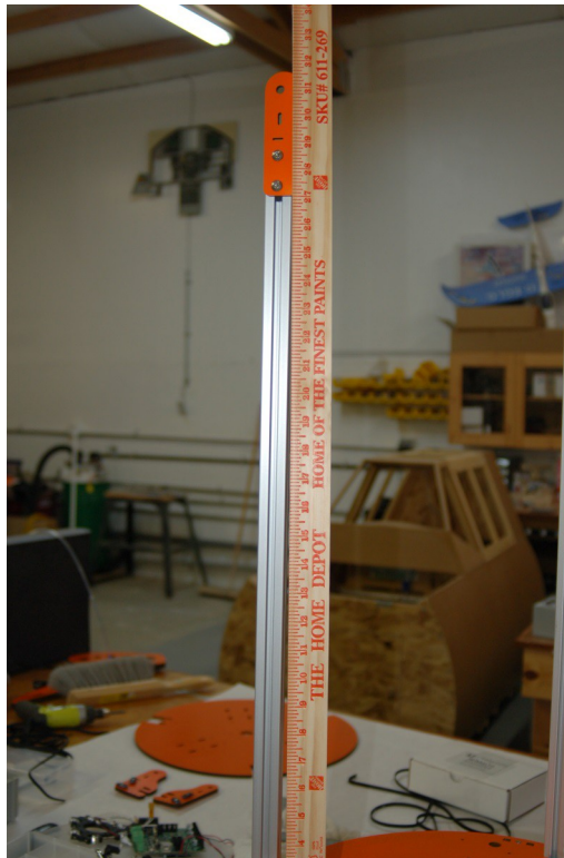
Fig. 4-3: Idler Mount spacing gauge.
