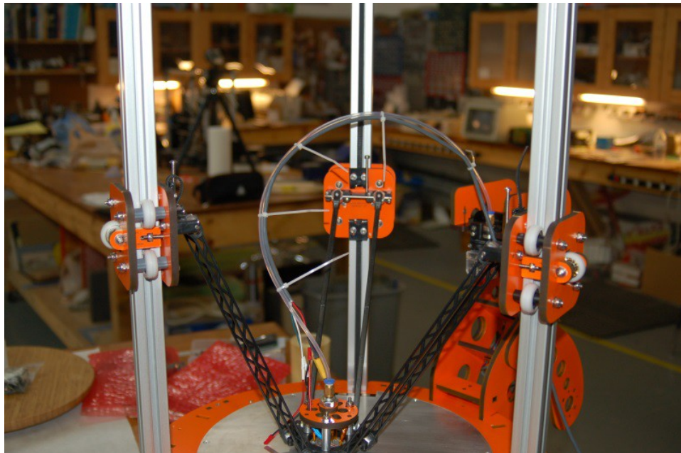
Fig. 16-9: Hot end wiring attached.
