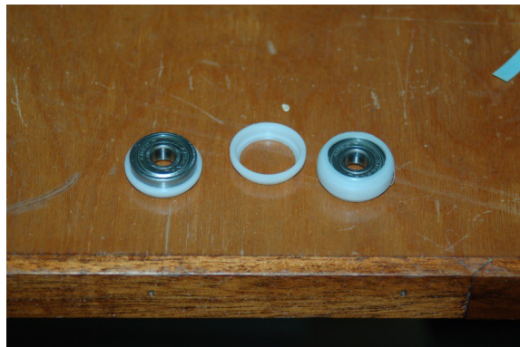
Fig. 7-2: Assembling the bearing covers
