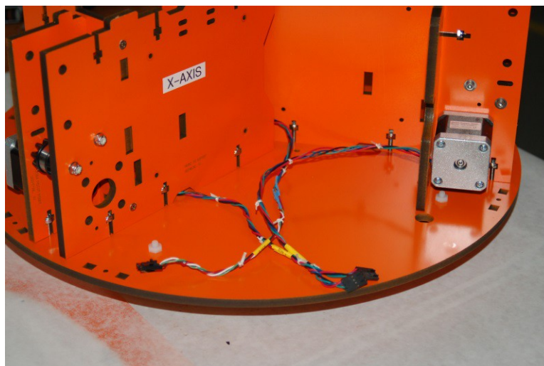
Fig. 2-30: Stepper motor wire routing.
