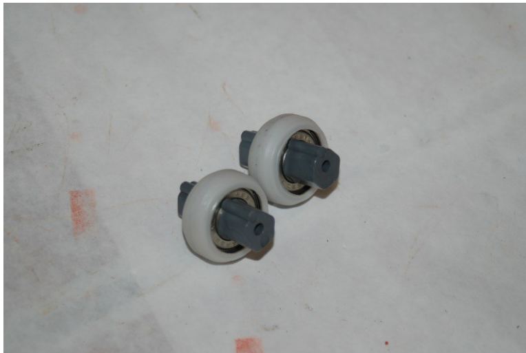
Fig. 7-17: Bearing assemblies with eccentric cams in place
