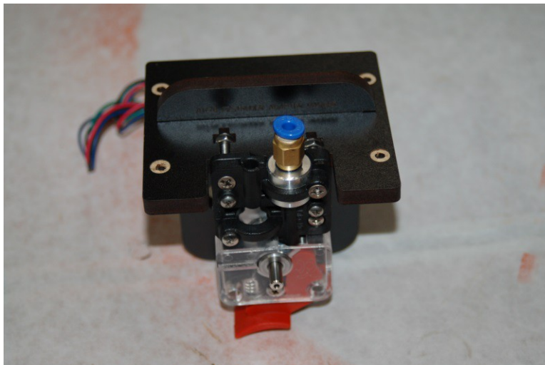
Fig. 12-13: EZStruder mounted to the adapter plate.
