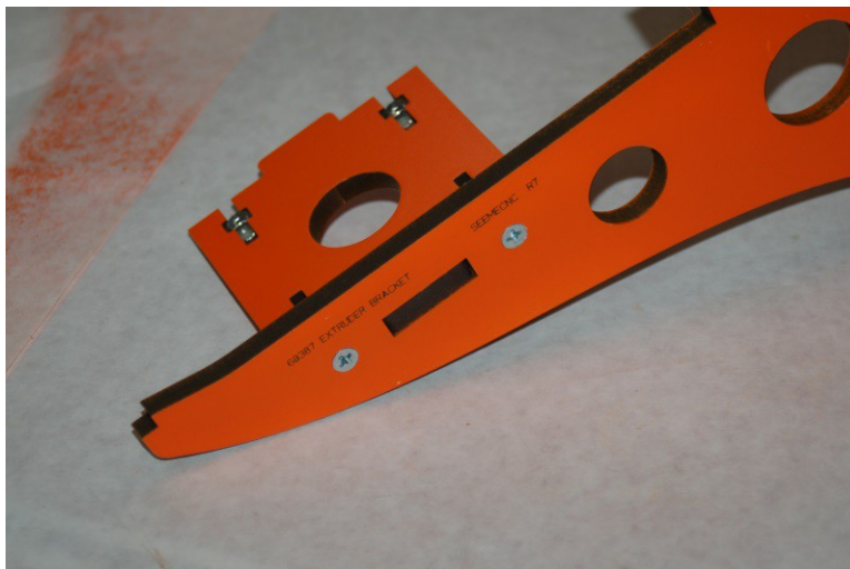
Fig. 11-4: Installing the first extruder support.
