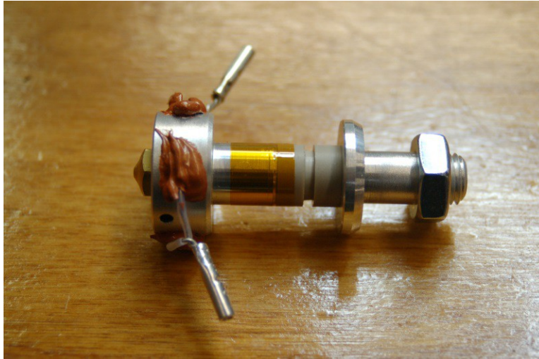
Fig. 15-6: Kapton wrap on the PEEK barrel.
