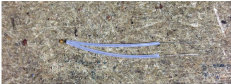
Fig. 3-5: Thermistor with PTFE sleeves installed.
