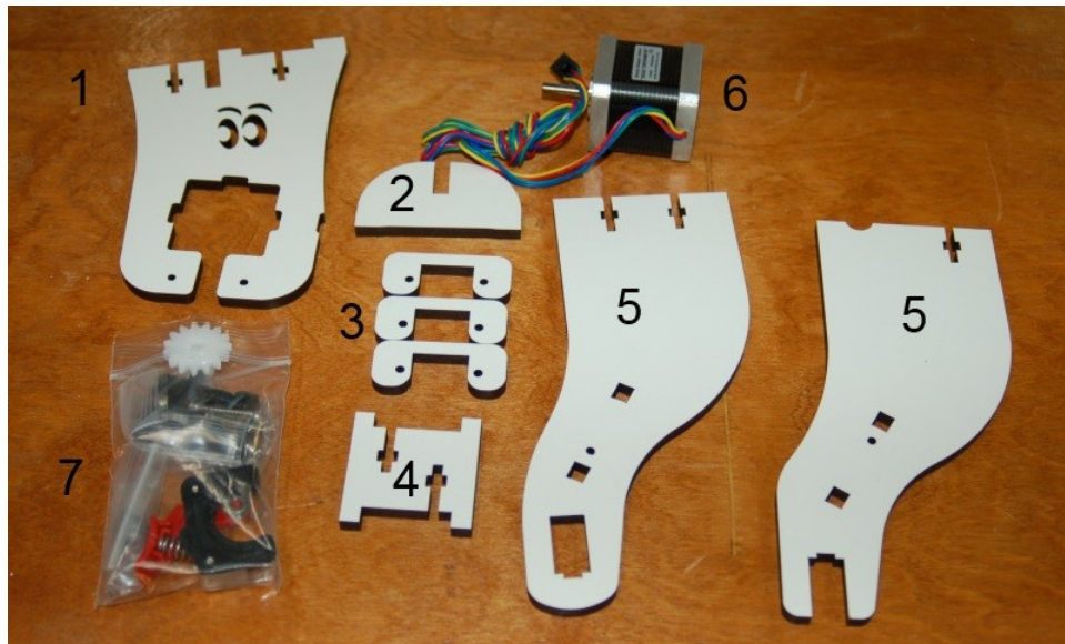
Fig. 12-1: EZStruder & Filament Holder Components.
