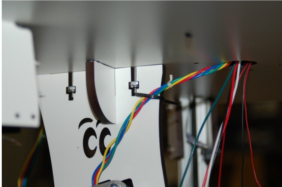
Fig. 12-14: Routing the extruder wires.
