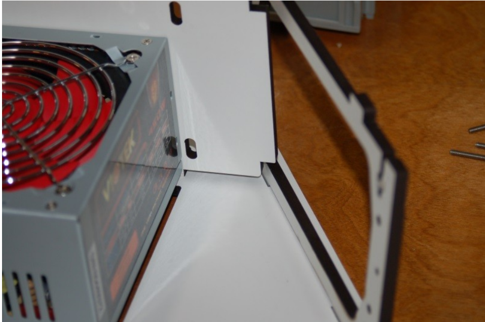
Fig. 4-12: Detail of power supply bracket, right side.
