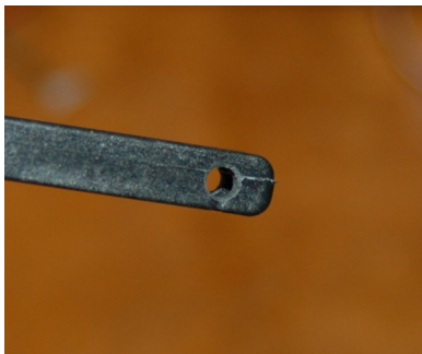
Fig. 14-6: Cleaned arm tips.
