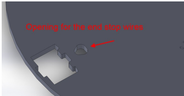
Ill. 10-1:End-stop wire routing hole.
