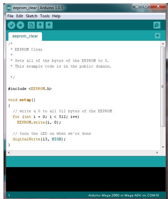
Fig. 20-5: eeprom_clear loaded and ready to go.
