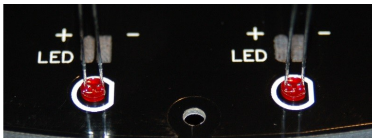
Fig. 5C-12: Power LED orientation.
