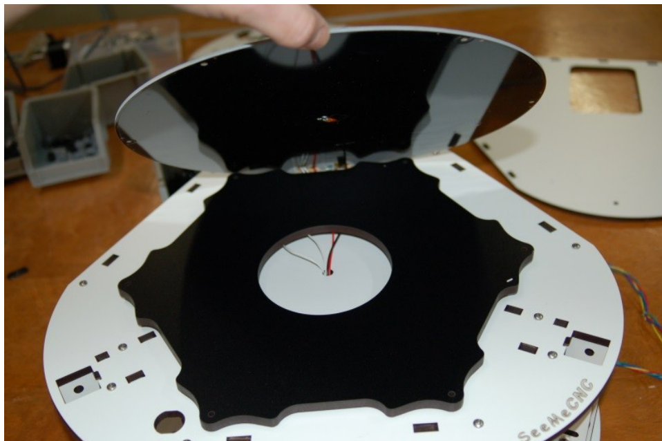
Fig. 5A-15: Orienting the Onyx on the mounting plate.
