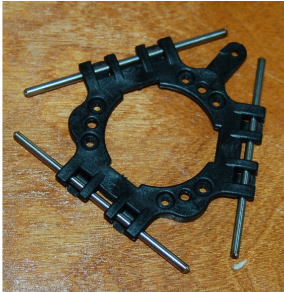
Fig. 14-2:U-Joint axles installed.
