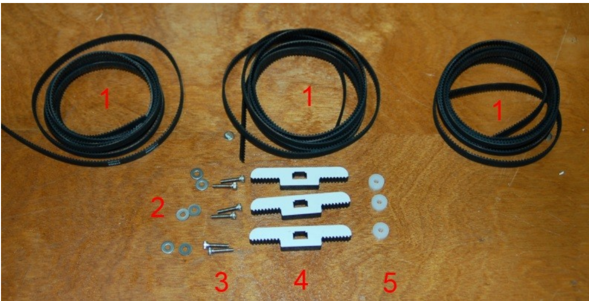
Fig. 11-1: Belt Clamp Components.
