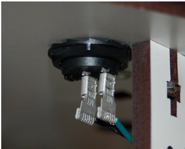
Fig. 18-31:Power switch installed.
