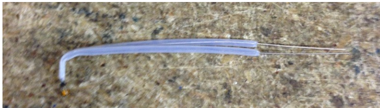
Fig. 3-6: Bending the thermistor.
