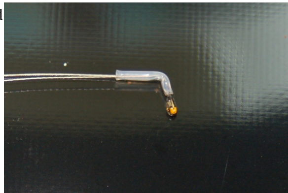
Fig. 5A-3: Thermistor properly bent.
