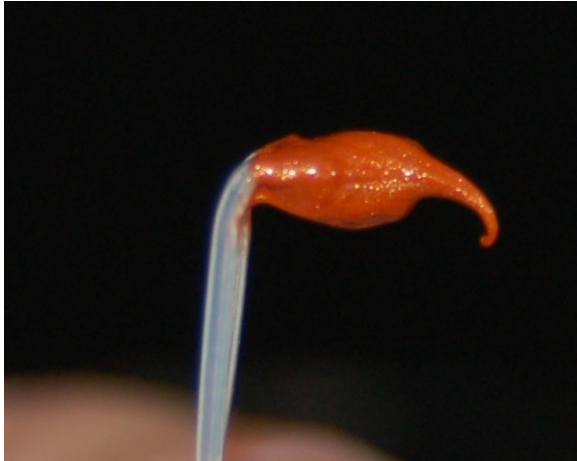
Fig 5C-6: Thermistor dipped in RTV.
