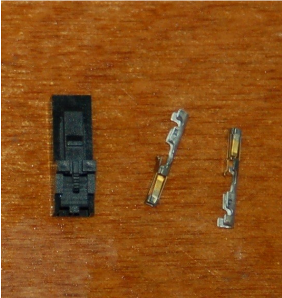
Fig. 18-10:2 pin female connector and crimp pins.
