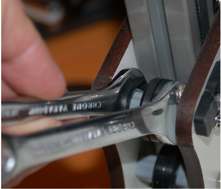
Fig. 8-28: Adjusting the eccentric spacers.
