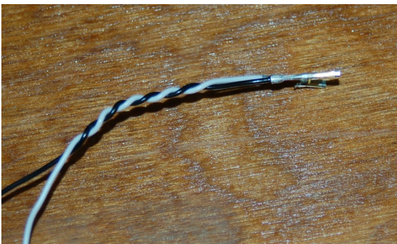
Fig. 6-8: Spindled wire ends.
