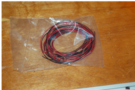
Fig. 6-4: 26ga wire for fans.
