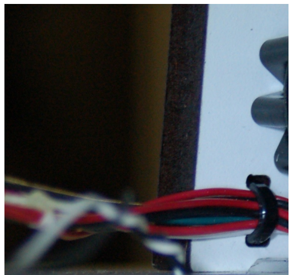
Fig. 10-12: Tie-down point, inside face.
