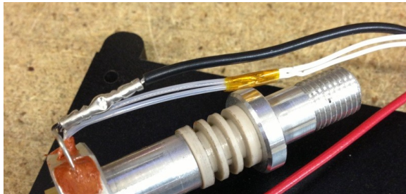
Fig. 13-15: Thermistor lead routing.
