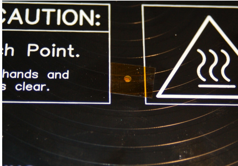
Fig. 5C-4: Covering the thermistor hole.
