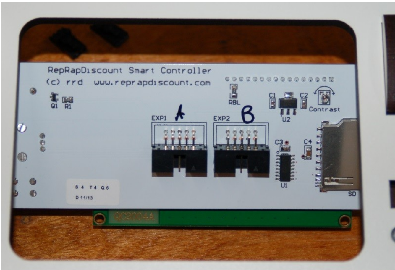
Fig. 17-12: Marking the interface connectors.
