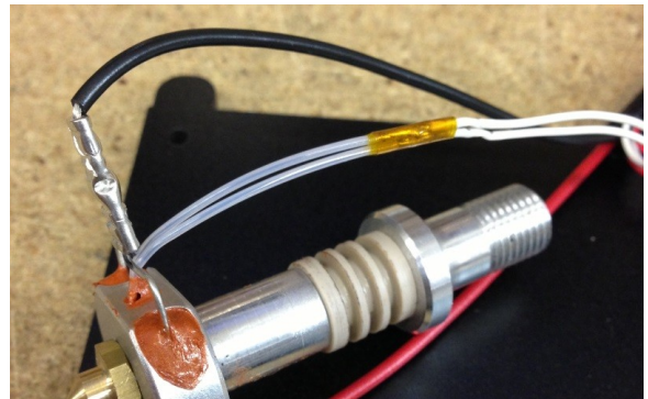
Fig. A-19:Kapton covered leads.
