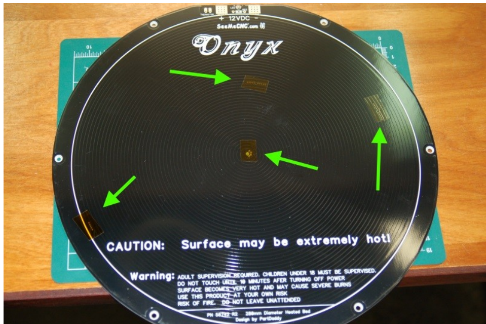
Fig. 5A-2: Via locations that need to be covered.
