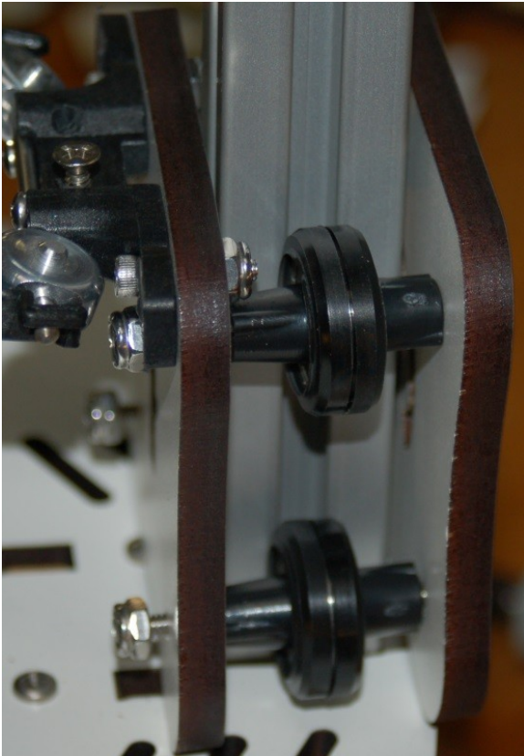
Fig. 8-25:Installing the #6-32 nuts.
