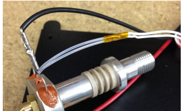
Fig. 13-16: Kapton covered leads.
