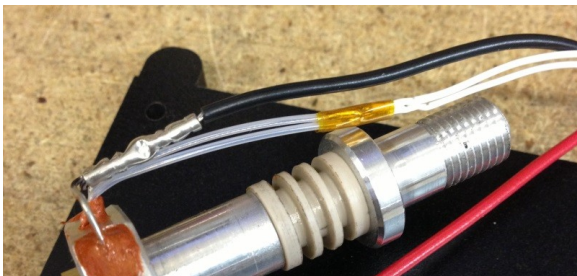
Fig. A-20:Thermistor lead routing.
