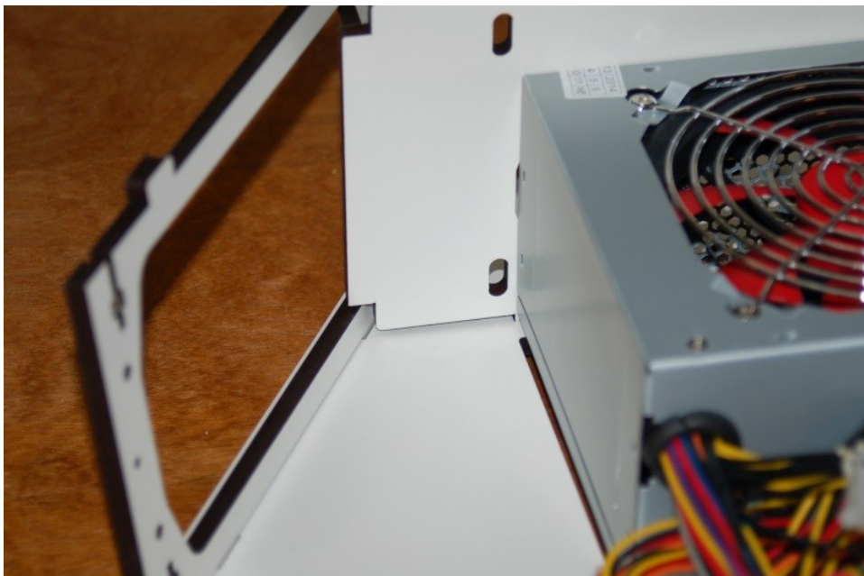
Fig. 4-13: Detail of power supply bracket, left side.
