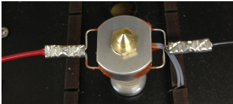
Fig. A-15: Power wires connected.
