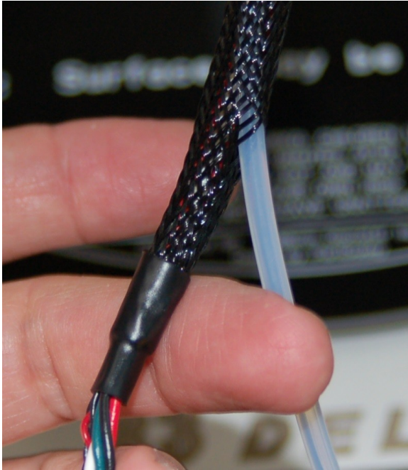
Fig. 13-22: Inserting the bowden tube.
