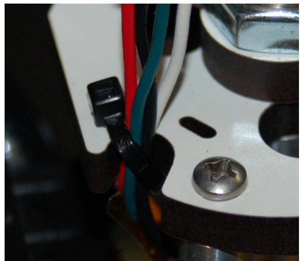
Fig. 13-21: Wire tie detail.
