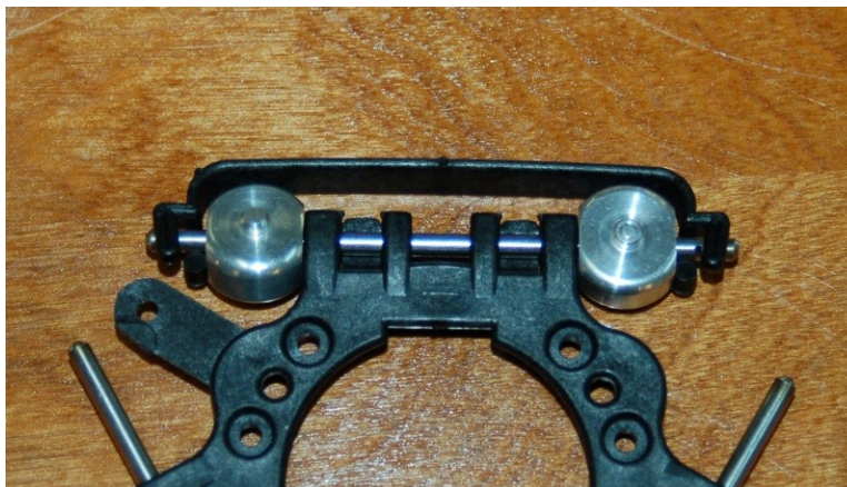
Fig. 14-3:U-Joints and spring clip installed.
