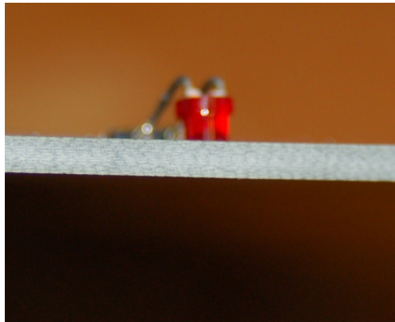
Fig. 5C-16: Correct LED depth.
