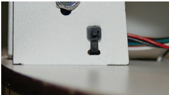
Fig. 10-11: Tie-down point, outside face.
