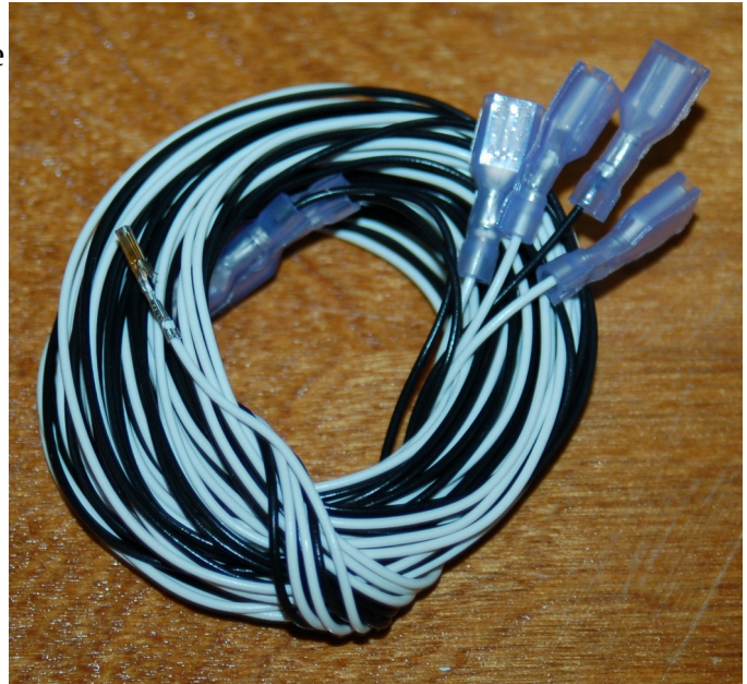
Fig. 6-7: End stop wires.
