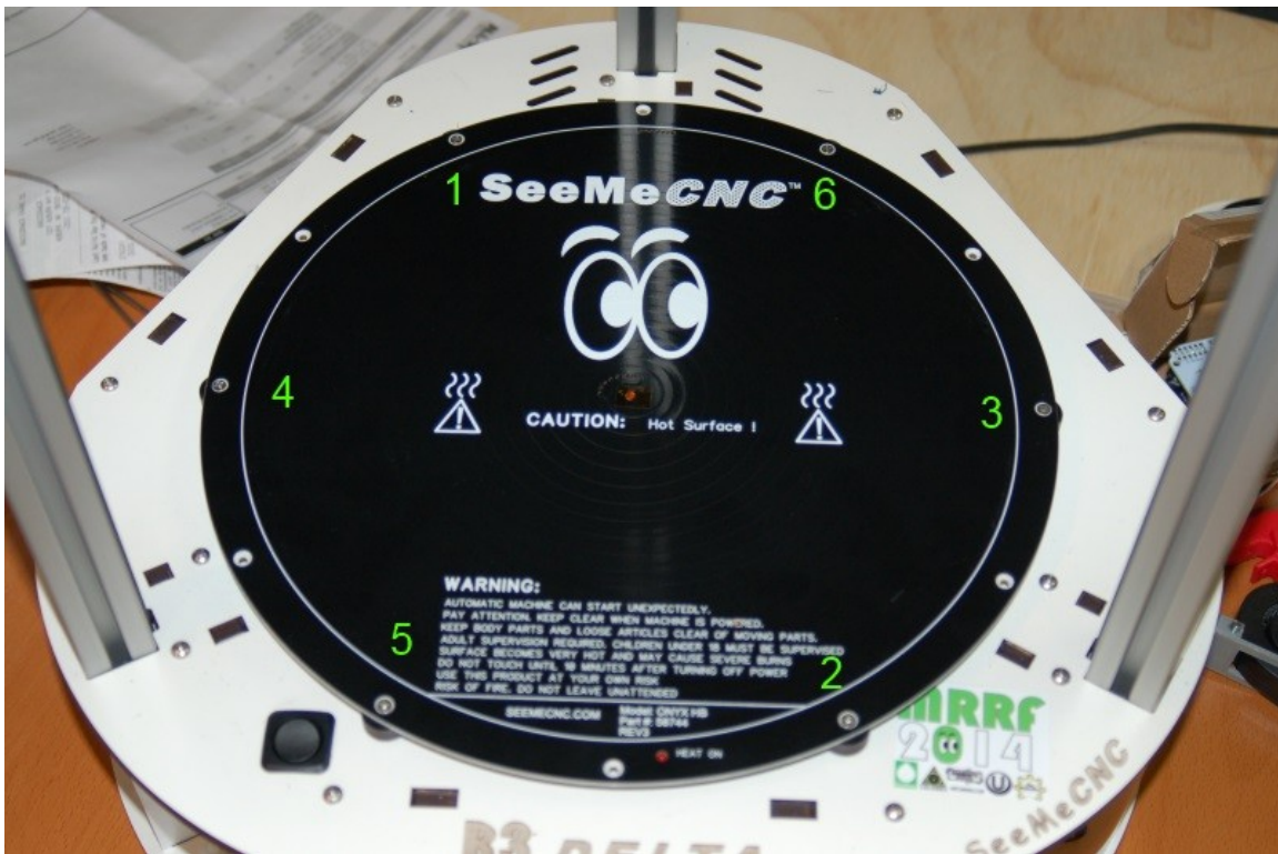
Fig. 5B-25: Screw tightening pattern
