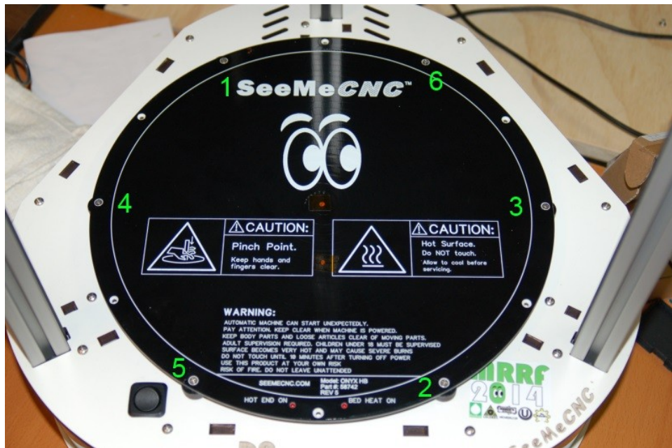
Fig. 5C-29: Screw tightening order.
