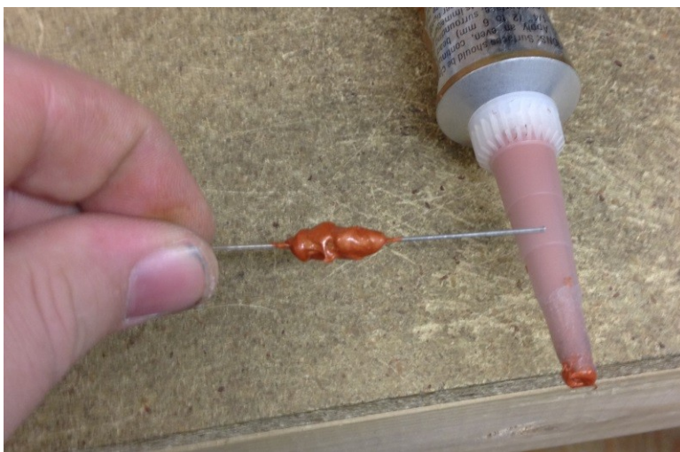
Fig. 3-2: Coating the heating resistor with RTV.
