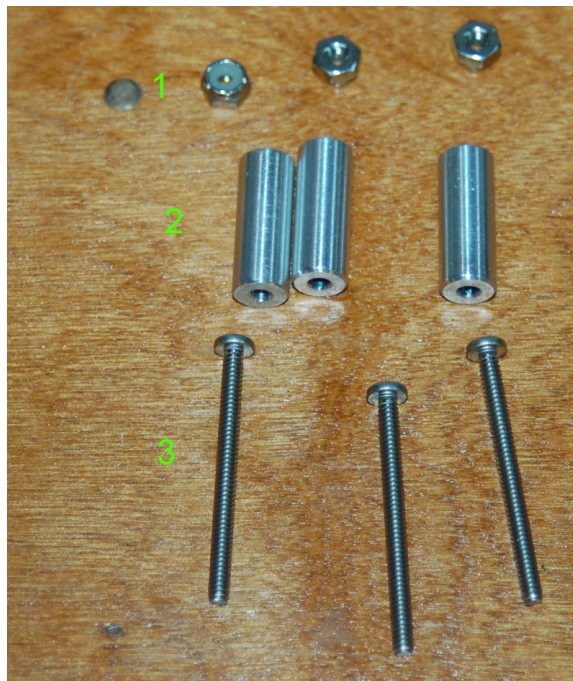
Fig. 15-1: Hot End Mounting Hardware.
