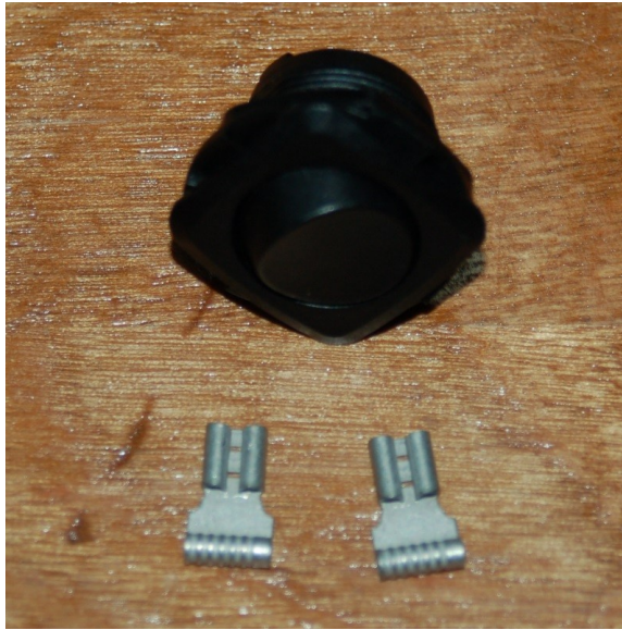
Fig. 3-10: Power switch and crimp-on spade lugs.
