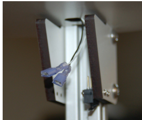
Fig. 8.7-2: Z axis wires ready to plug in.
