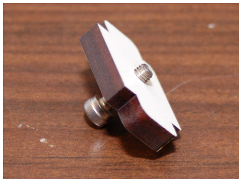
Fig. 8.1-2: Threading the spacers.
