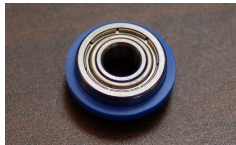
Fig. 9.1-2: Pressed into the sleeve.
