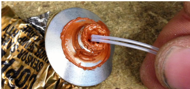
Fig. 3.1-8: Coating the thermistor with RTV.
