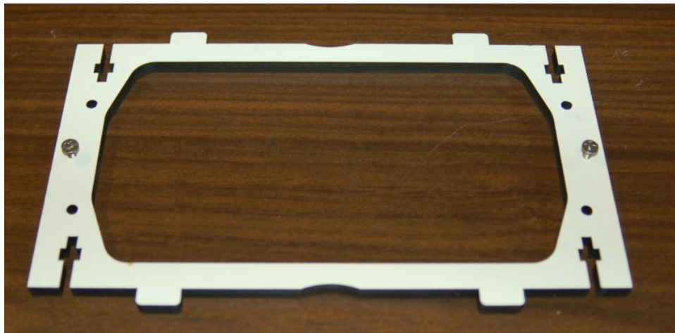
Fig. 6.2-3: Vertical support with panel retaining screws installed.
