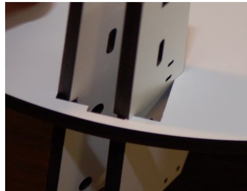
Fig. 8.2-2: Right mount in the correct position.
