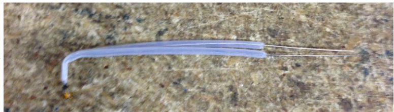
Fig. 3.1-7: Bending the thermistor.
