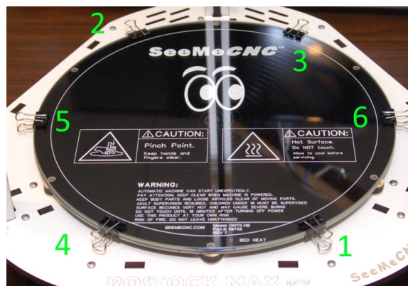
Fig. 18.4-4: Document clips installed.
