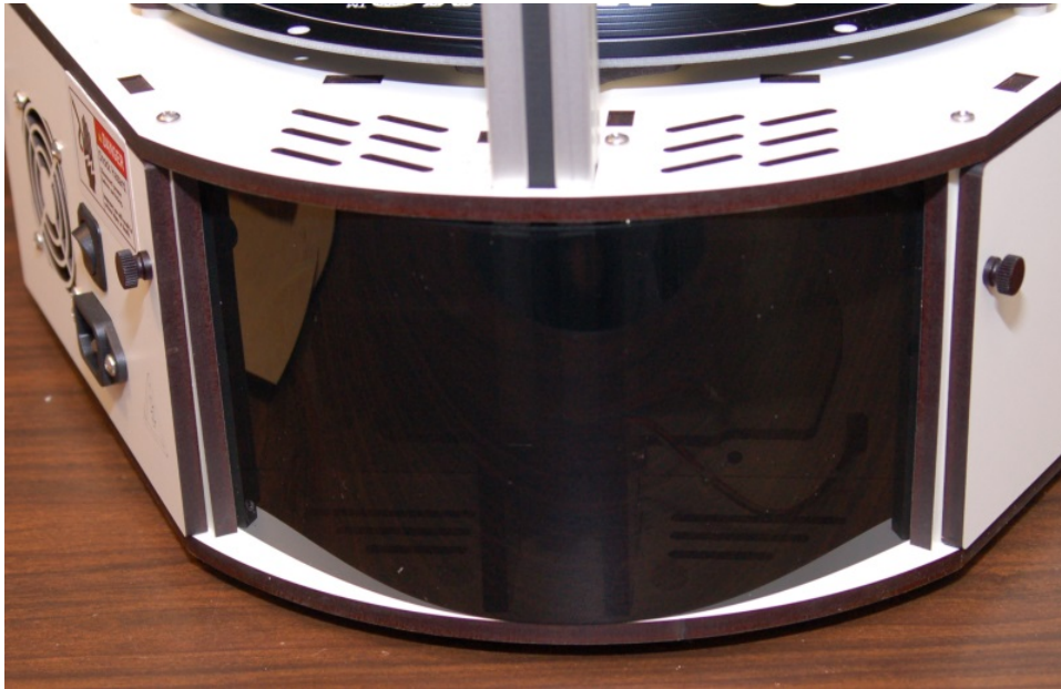
Fig. 18.3-3: Z Axis cover installed.
