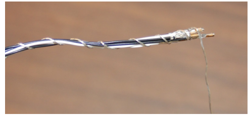
Fig. 7.1-6: End-stop wires ready to pull.
