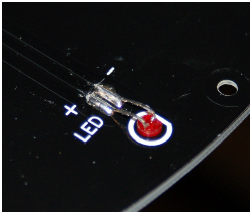
Fig. 4.2-5: Soldered and trimmed!
