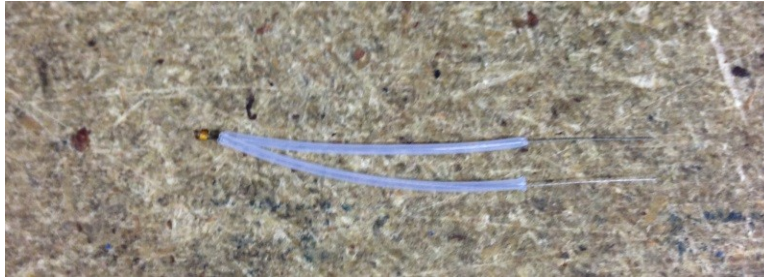
Fig. 3.1-6: Thermistor with PTFE sleeves installed.
