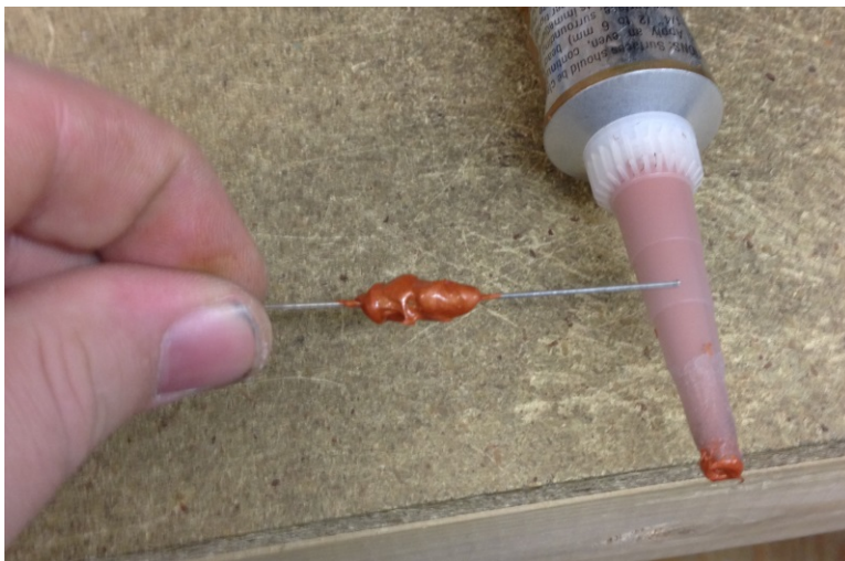
Fig. 3.1-3: Coating the heating resistor with RTV.
