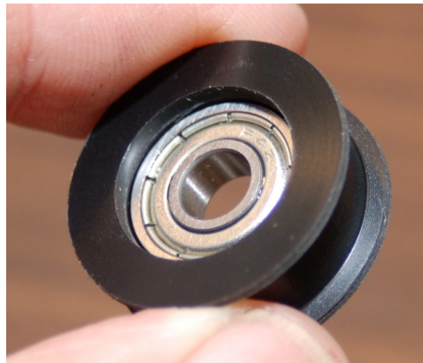
Fig. 6.7-2: R4 bearing installed.
