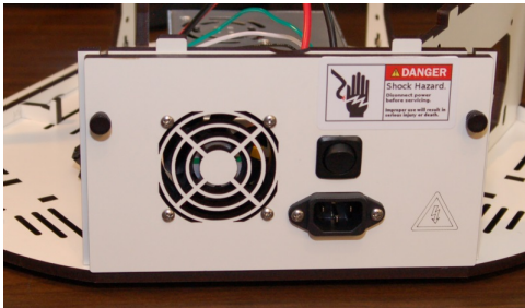
Fig. 6.6-8: Power supply install complete.
