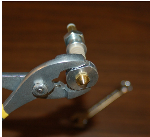
Fig. 3.1-1: Tightening the nozzle.
