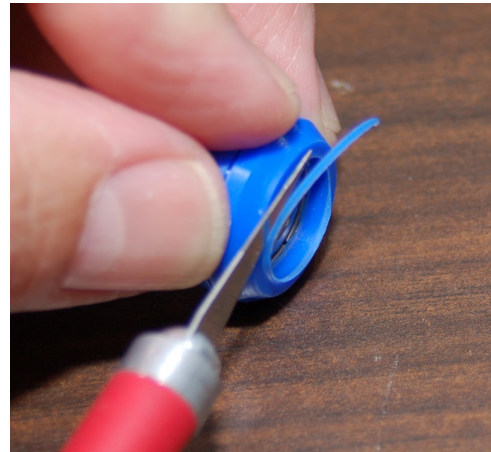
Fig. 9.1-5 Removing the edge.
