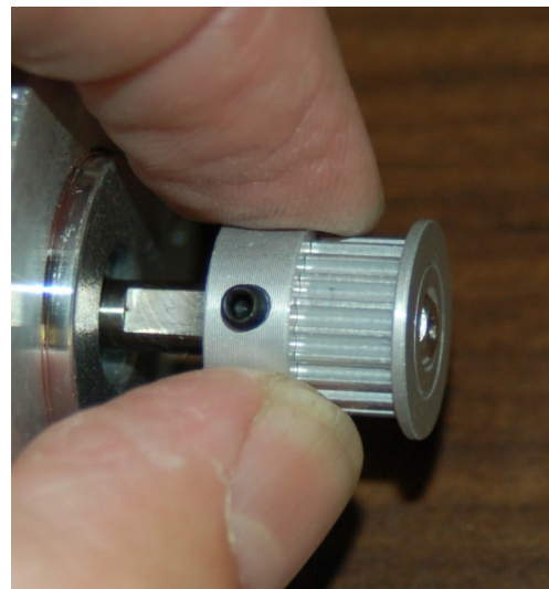
Fig. 5.1-2: Gear and grub screw aligned.
