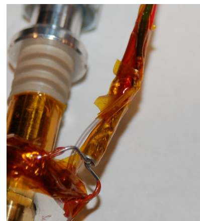
Fig. 11.3-12: Thermistor leads bound tight. (Older wire style shown.)
