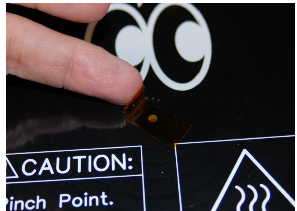
Fig. 4.1-1: Covering the thermistor hole.
