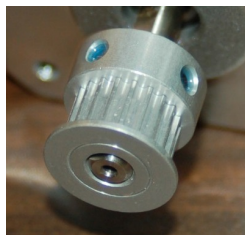
Fig. 5.1-3: Drive gear installed.
