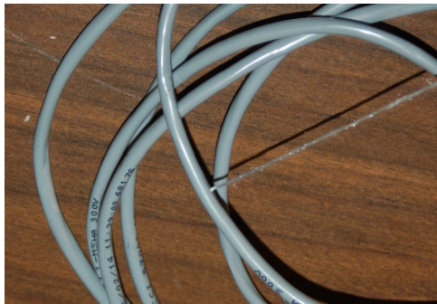
Fig. 7.1-1: Splitting the outer jacket.
