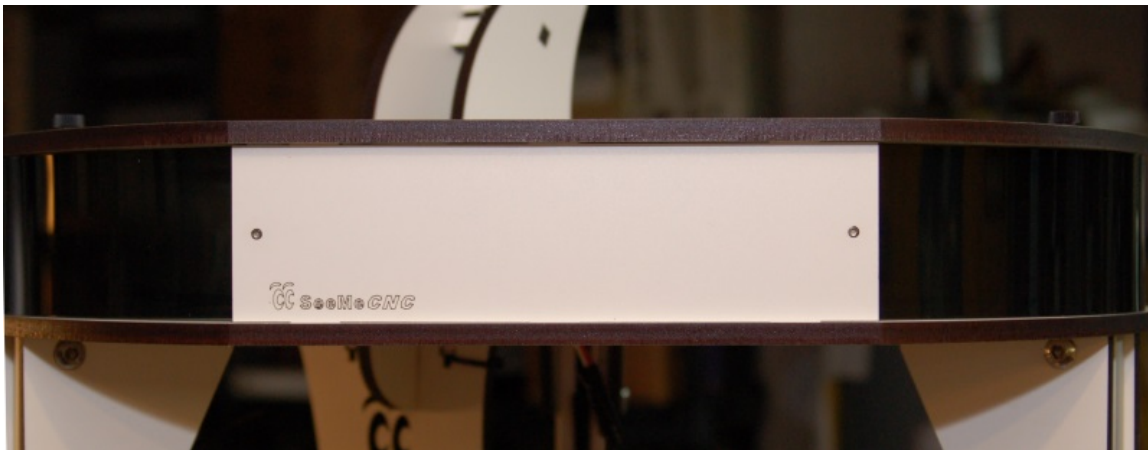
Fig. 18.3-4: Upper acrylic covers installed.
