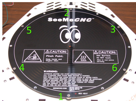
Fig 15.1-5: Screw tightening pattern.
