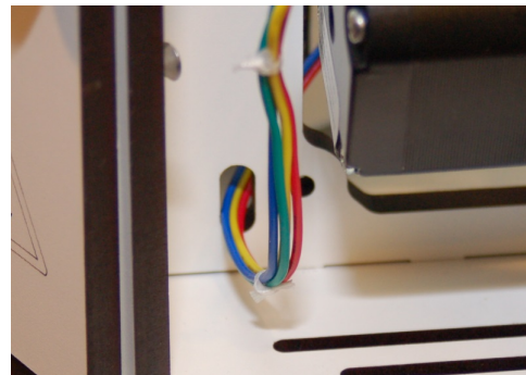
Fig. 6.8-2: Z Axis motor wire route.
