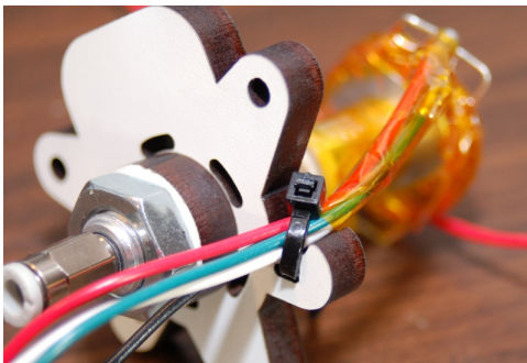
Fig. 11.4-3: Wires fixed in place.
