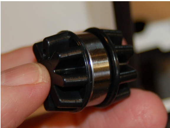
Fig. 7-19: Upper idler bearing.
