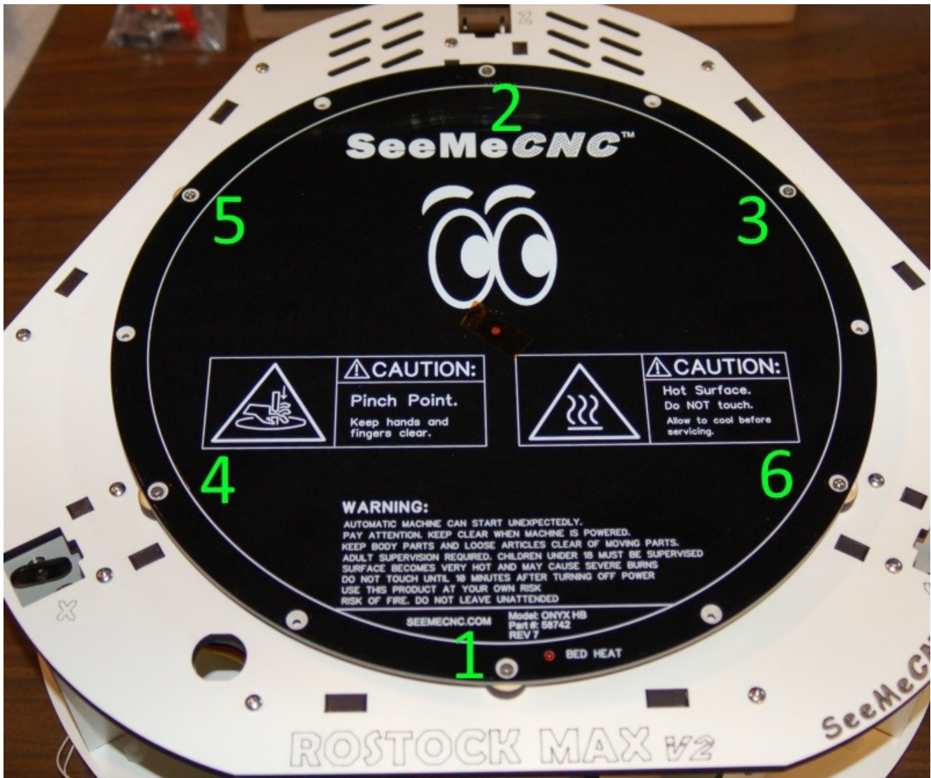
Fig. 5-32: Screw fastening order.
