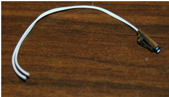
Fig. 16-19: Thermistor leads cut to length.
