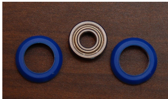
Fig. 8a-1: R4ZZ bearing and two sleeve halves.
