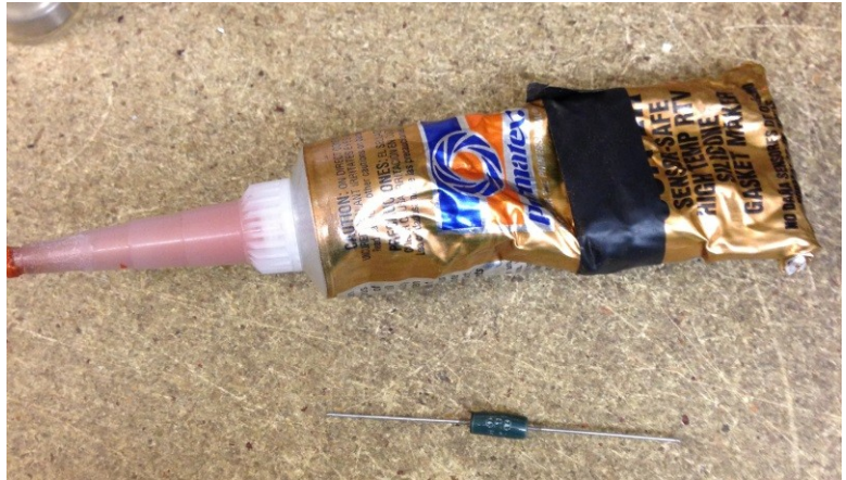
Fig. 3-2: RTV & heating resistor.
