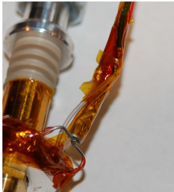
Fig. 11-20: Thermistor leads bound tight.
