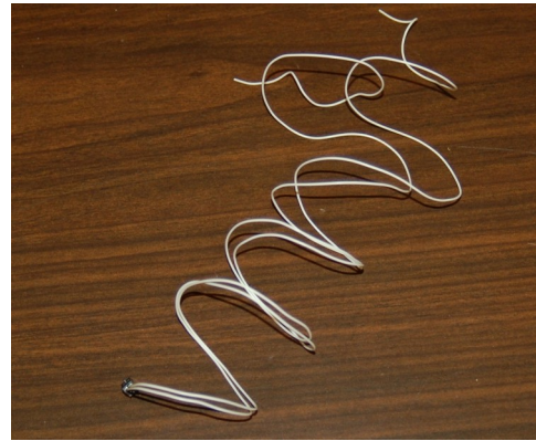
Fig. 5-22: Single thermistor signal lead.
