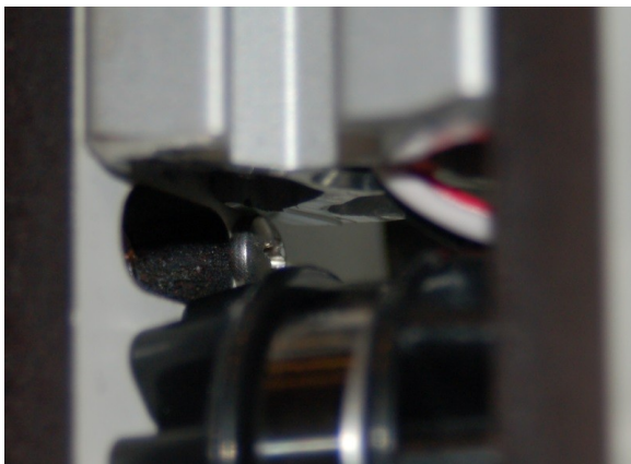
Fig. 6-17: Tower fully seated, resting against the stop screw.
