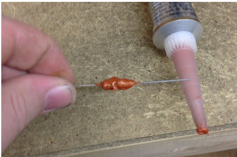
Fig. 3-3: Coating the heating resistor with RTV.
