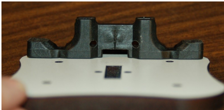
Fig. 8-7: U-Joint carriage fitted properly.
