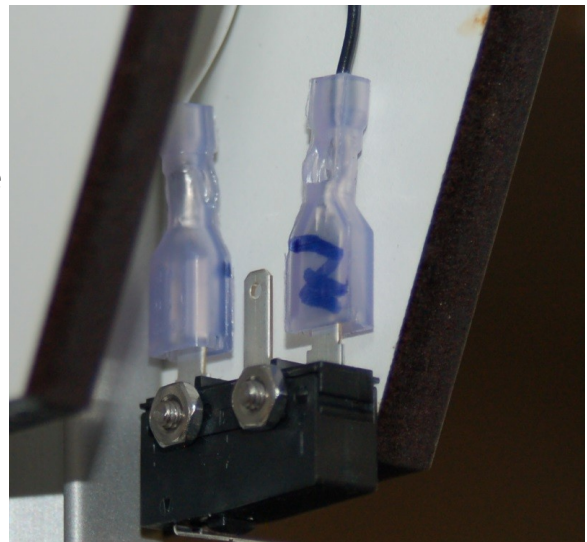
Fig. 7-34: Z axis end stop switch wired.
