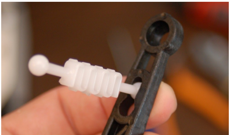
Fig. 12a-6: Example Ball-End Tension Spring installation.
