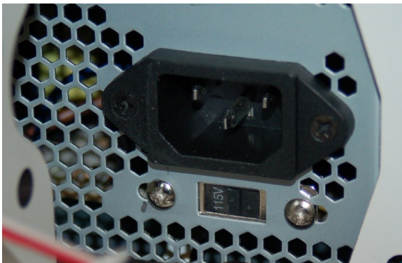
Fig. 17-5: Source voltage switch.
