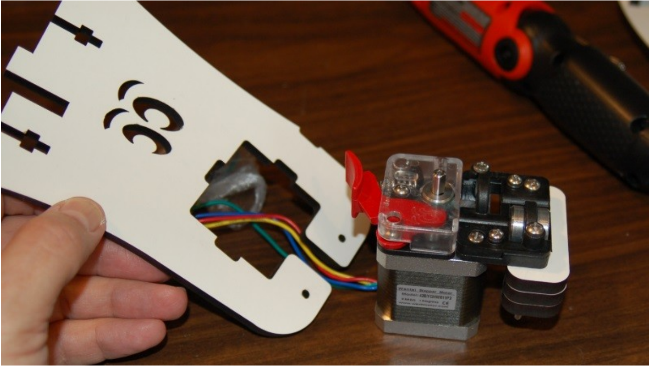
Fig. 10-13: Bracket & EZStruder orientation.
