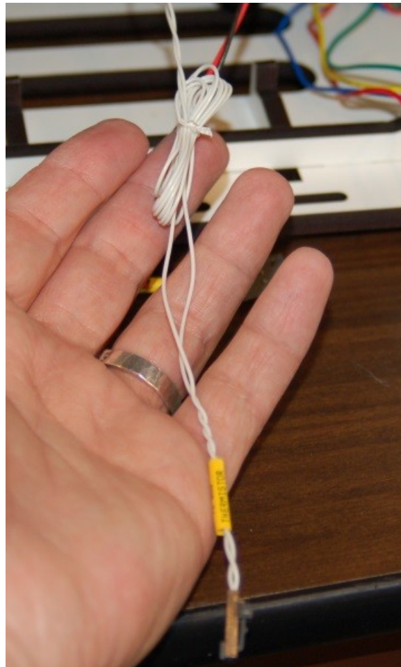
Fig. 16-23: Bed thermistor wire bundled up
