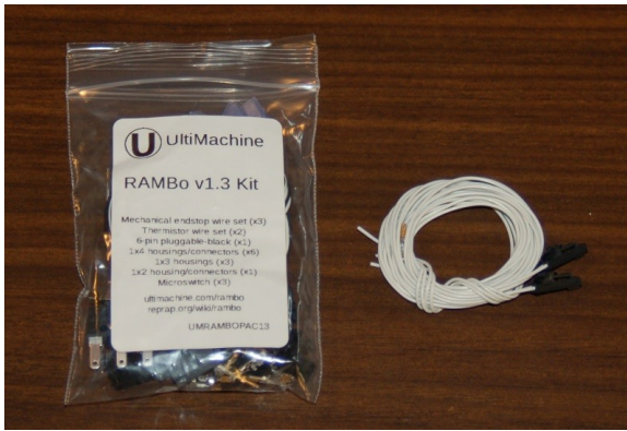
Fig. 5-21: Thermistor wire bundle.
