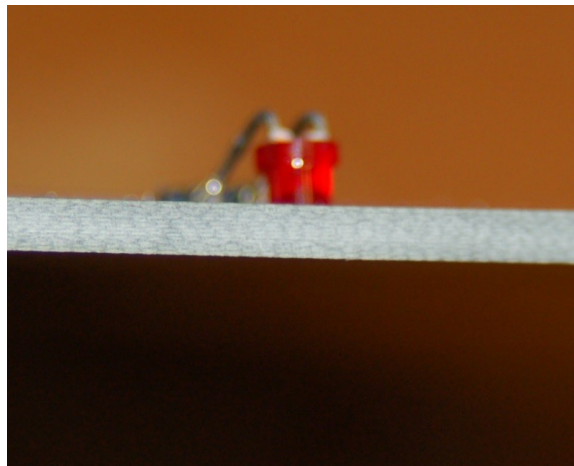
Fig. 5-13: Correct LED depth.
