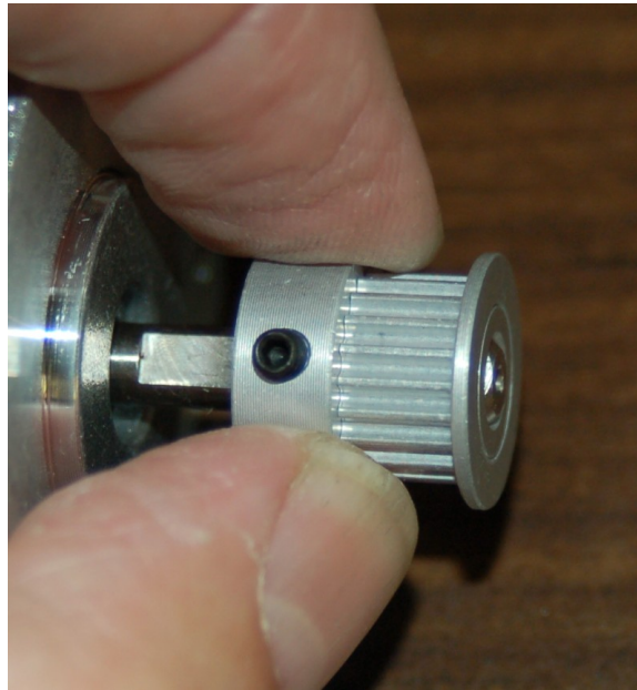
Fig. 4-27: Pulley & grub screw aligned.
