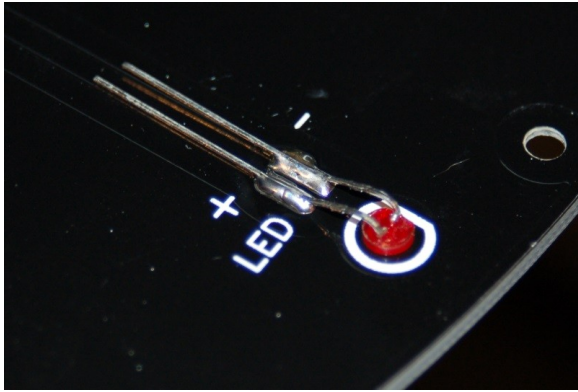
Fig. 5-11: Leads soldered into place.
